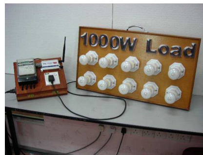
Fig. 5. GSM Power Meter and 1000W Load for Demonstration
