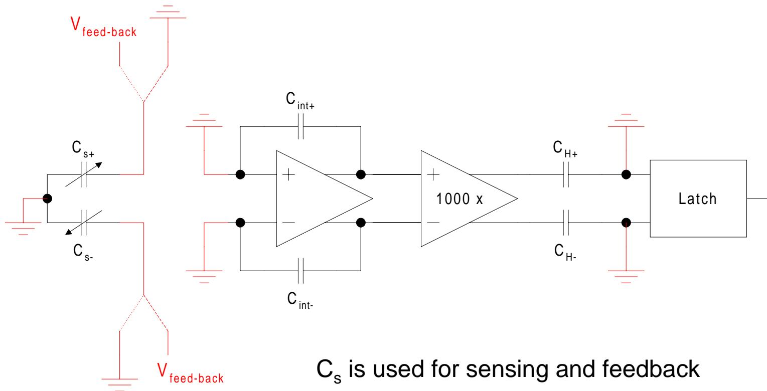
$C_s$  is used for sensing and feedback
