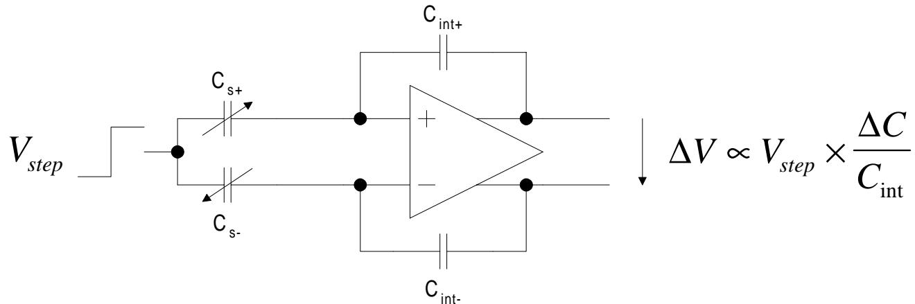
$$\Delta V \propto V_{step} \times \frac{\Delta C}{C_{int}}$$
