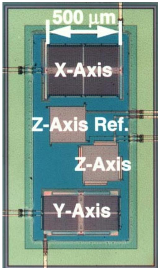
Ref.: M. Lemkin et al., "A 3-axis surface micromachined  $\Sigma\Delta$  accelerometer," in digest ISSCC, pp. 202-203, February 1997.
